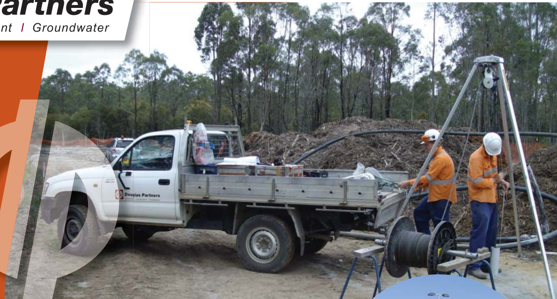
Douglas Partners deploying our in-house downhole sonars to further investigate the layout of the workings.
