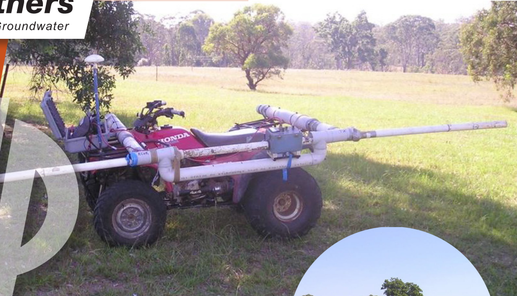
Quad bike fitted with Electromagnetic Profiler collecting data on site.
