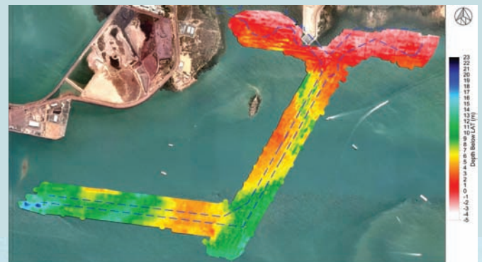
Above: Bedrock depths from seismic reflection Right: N-S refraction tomogram with bedrock reflection overlay
